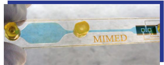
The MIMED system is a universal point-of-care pathogen detection system. The 6x1 cm disposable chip integrates sample preparation and sequence-specific detection and can identify microbes in unprocessed biological, water, food, and forensic samples.
