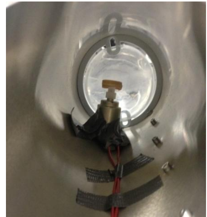
Figure 5: Inside view of ballpoint laparoscope with rotating motor mechanism.
