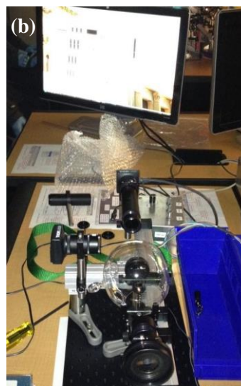
Figure 7: Optical rig set-up for testing resolution, light intensity, and contrast, using the glass sphere
