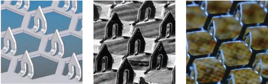
Figure 12: 12a-SolidWorks (CAD) depiction of microneedles, 12b-SEM image of microneedles, 12c-Actual photograph of microneedles
