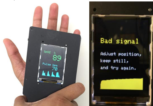
Figure 6 (left) The final output of Luminox on the LCD color screen. (right) An error message indicates a potentially erroneous reading.
