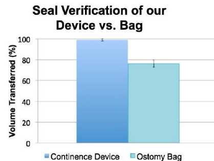
Figure 8: Bovine experiment testing bed (Left) and results from seal verification testing (Right)
