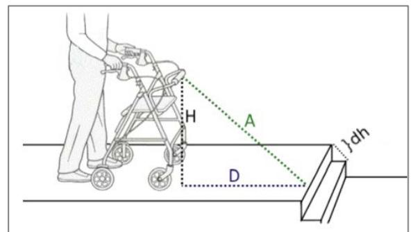
Figure 2. The sensors constantly sample the distance A, then A +dh. Length H is the top crossbar height of the patient's walker. Length D is the patient's safe stopping distance. For David, these are: H = 2.5' and D= 4.0'.
