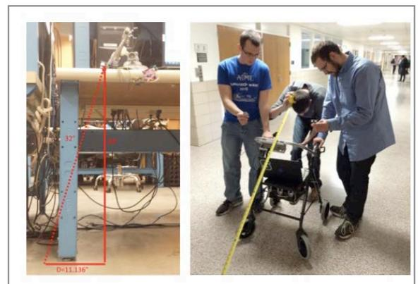
Figure 3. Angle of depression tests for all candidate sensor types proved critical to success. Shown: D. Hill, S. Moore and Y. Kochubievsky.
