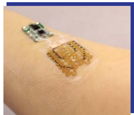
Smart wound dressing is thin and flexible with an array of pH sensors, thermo-responsive drug carriers, and an onboard controller. Source: Khademhosseini lab, Harvard-MIT.
