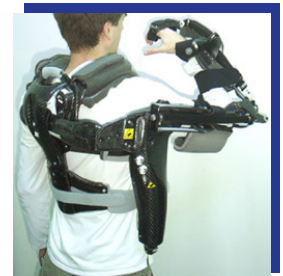
RUPERT: a device for robotic upper extremity repetitive therapy. Source: Jiping He, Arizona State University
