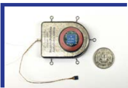
Wireless, implantable brain sensor, shown next to a U.S. quarter for size comparison. Source: David Borton, Ph.D., Brown University
