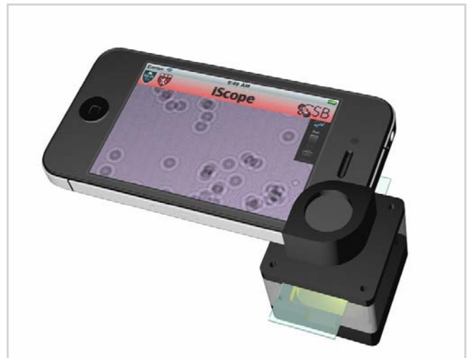
A cell phone with a special module can process cervical specimens to identify cancerous and precancerous cells. Credit: Ralph Weissleder and Hakho Lee/Massachusetts General Hospital.
