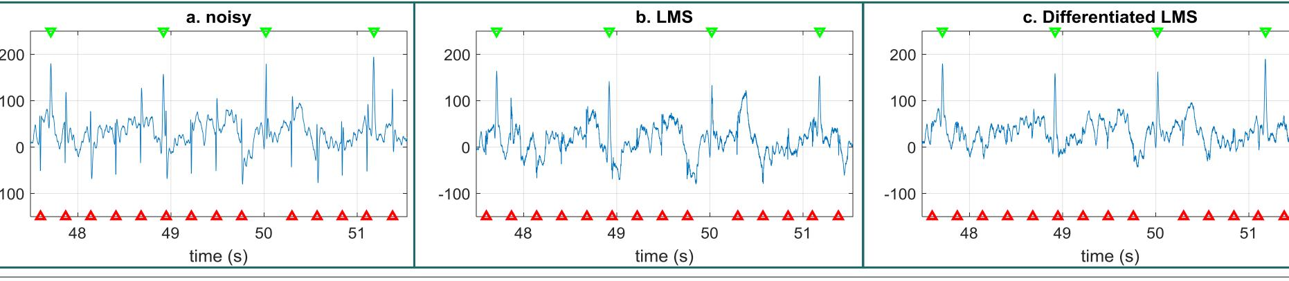
Fig 4. Left Leg ECG Signal distorted by MRI noise, and noise cleaned by adaptive filters. (a) Noisy, unfiltered signal. (b) The conventional Least Mean Squares (LMS) algorithm, currently in use by PRiME. (c) The differentiated LMS algorithm, a novel adaptive filter devised for this project. In both (b) and (c), three filters were used with one filter per unweighted reference signal.
