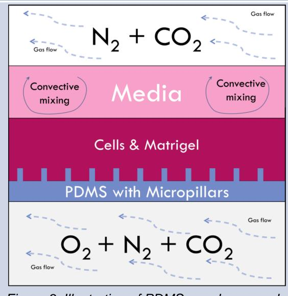
Figure 3. Illustration of PDMS membrane and cell culture material separating the top and bottom chambers.
