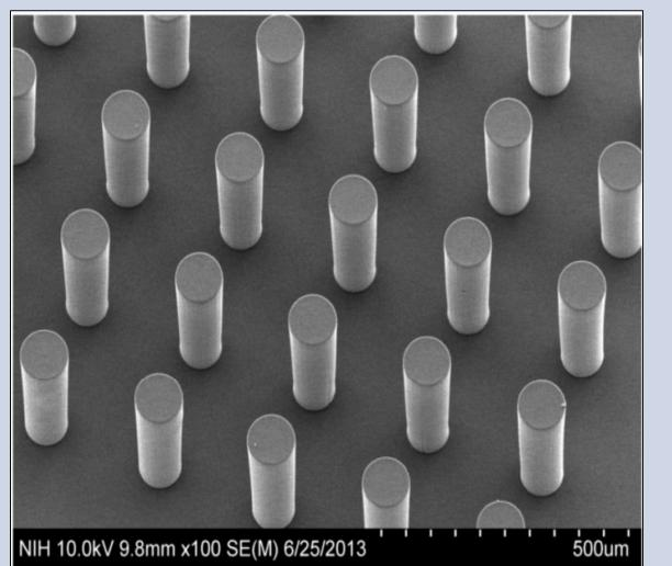
Figure 1. Scanning electron microscopy image of micropillars [5].
