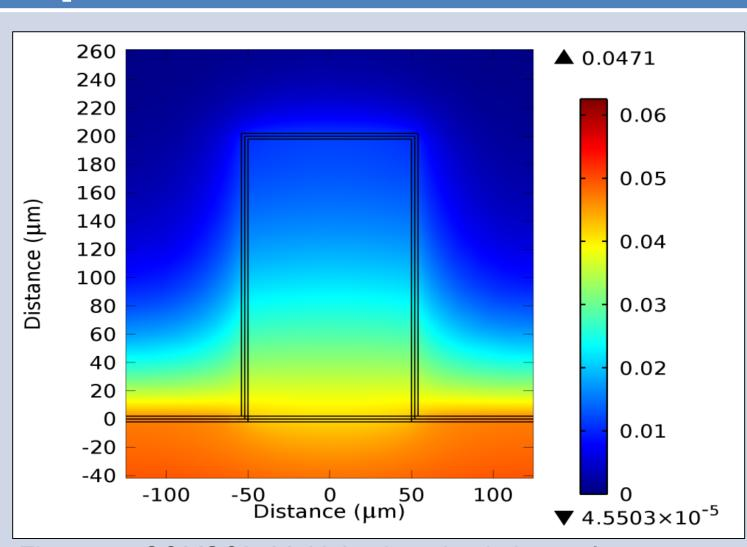
Figure 2. COMSOL Multiphysics simulation software modeling of oxygen gradient around a micropillar [5].
