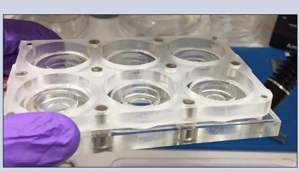
Figure 4. Image of custom 6-well plate with PDMS membrane.
