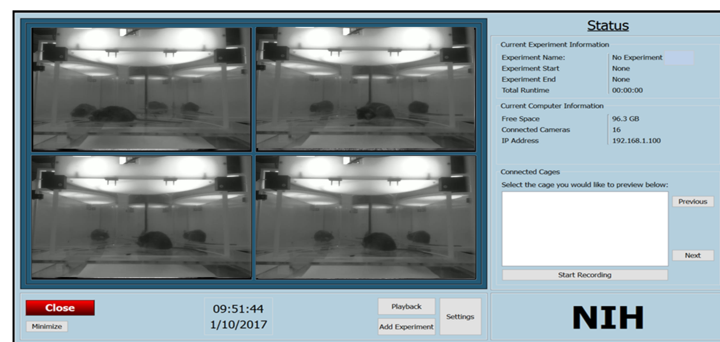
Python-based GUI for real-time video acquisition from the Raspberry Pi's camera of the arena to monitor the mouse's response to the administered itch drug.
