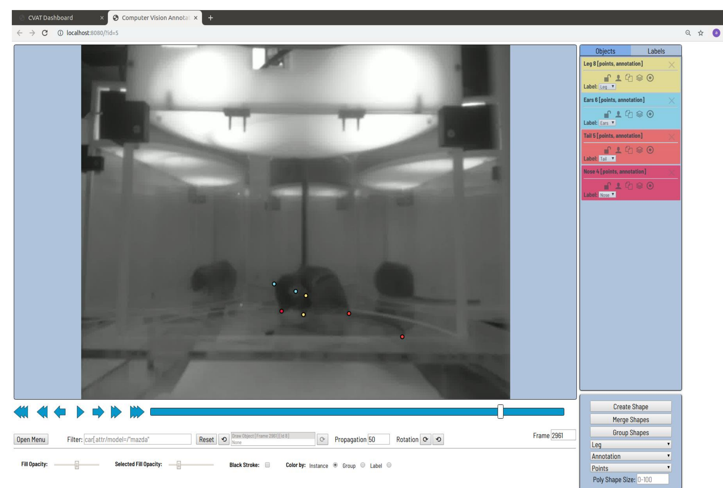
CVAT annotation software powered by OpenCV to create test data for machine learning algorithms. This is done by splitting the video into separate frames and annotating key attributes of the mouse such as ears, nose, hind legs, and tail.
