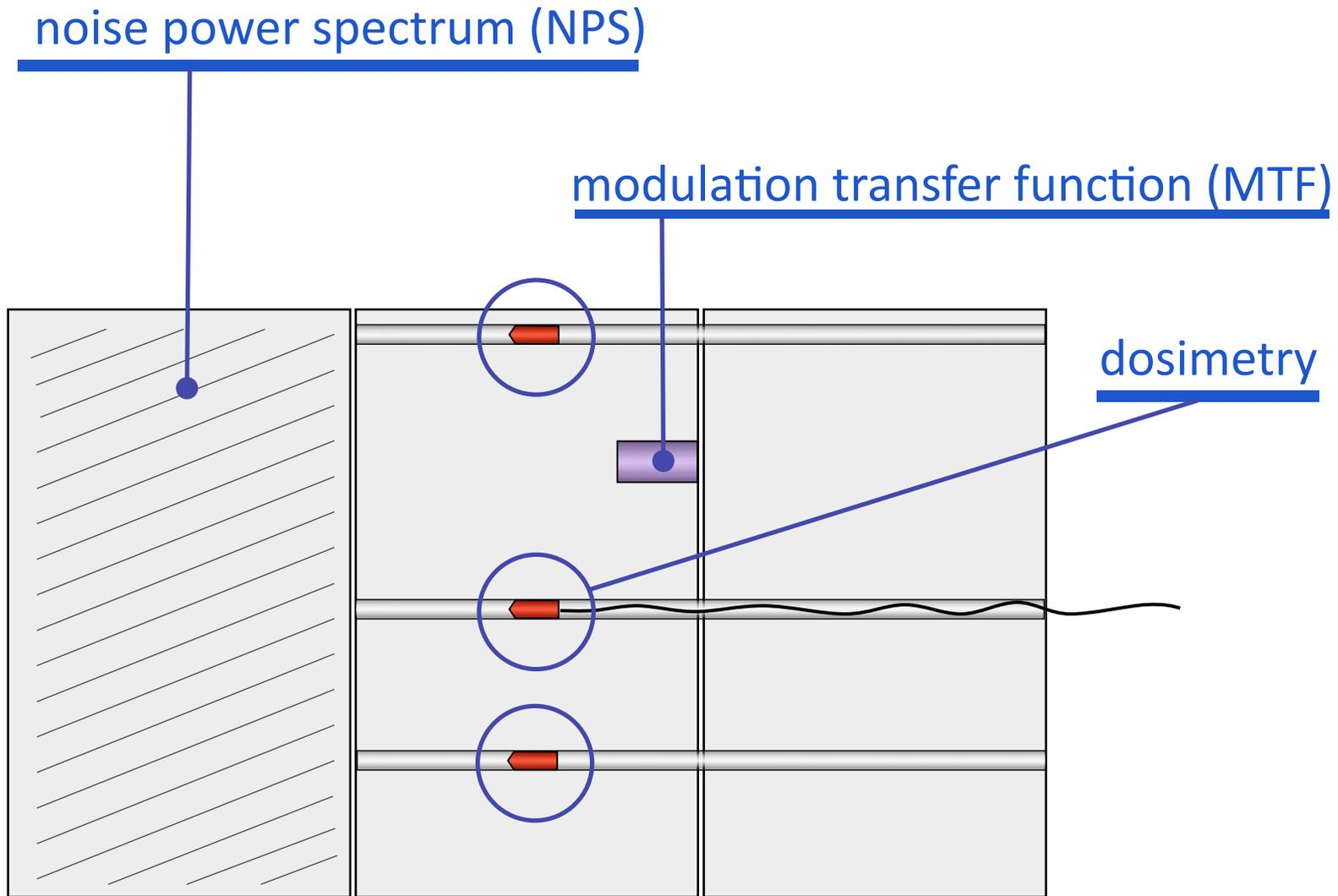
An Integrated CT Image Quality / Dosimetry Phantom
