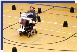
A man guides his wheelchair around an obstacle course using the tongue magnet and headset system. Source: M. Ghovanloo, Georgia Institute of Technology
