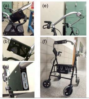
Figure 5. (a) Power supply housing, (b) battery life indicator, and (c) ANKER power supply in housing. (d) Fabricated crossbar and housing, and (e) Team Four final prototype.
