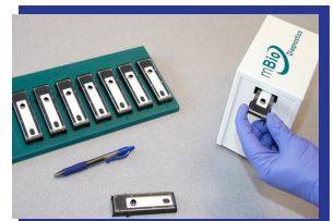
This low-cost, disposable cartridge system is used by minimally trained health workers in the field to simultaneously test blood samples for multiple infections. Results can then be interpreted, remotely, by health care experts.
