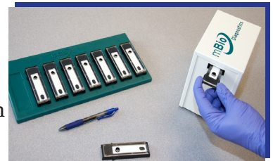
This low-cost, disposable cartridge system is used by minimally trained health workers in the field to simultaneously test blood samples for multiple infections. Results can then be interpreted, remotely, by health care experts. Source: Michael Lockhead, mBioDiagnostics
