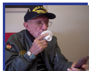
The patient breathes into the wireless capnograph, which sends breath patterns to the users phone where they are transmitted from home to a health care professional for evaluation. Source: Erica Forzani, Arizona State University
