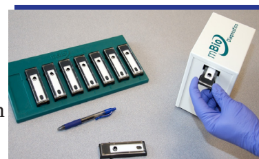
This low-cost, disposable cartridge system is used by minimally trained health workers in the field to simultaneously test blood samples for multiple infections. Results can then be interpreted, remotely, by health care experts. Source: Michael Lockhead, mBioDiagnostics
