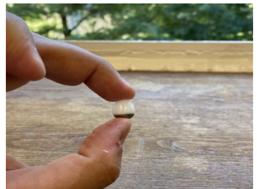
A robotic pill that can deliver biological drugs into the stomach lining. Usually these drugs require a shot. Credit: Giovanni Traverso
